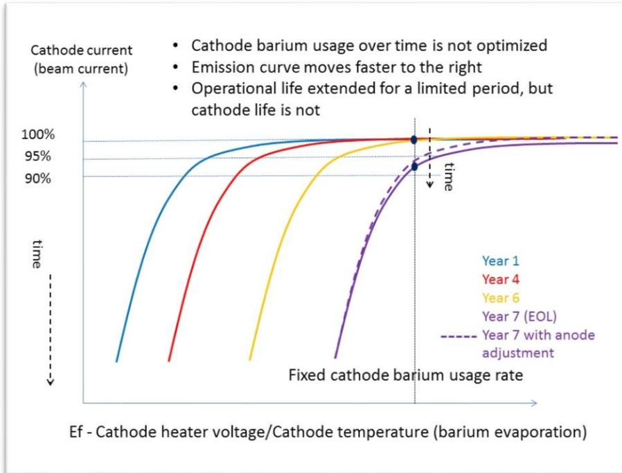
**Figure 1. This graph shows barium usage when heater voltage is fixed over time, as represented by the vertical black line. Except for years six and seven, the cathode's barium coating is burned off without being utilized efficiently.**
