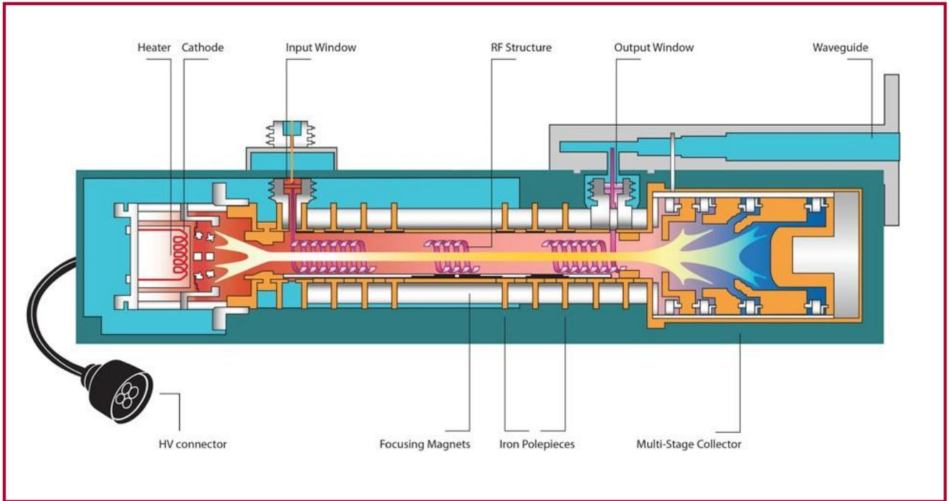
**Figure 3. Cross section of traveling wave tube. The cathode and heater at the left.**
